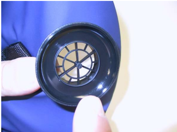
Clean the valve seat and check that the valve seat is ok
