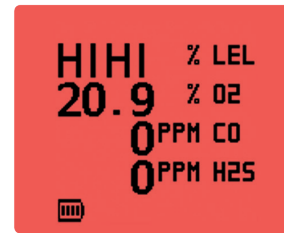
Red display in alarm conditions
