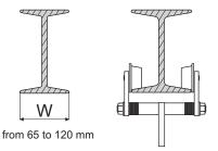
3. Make sure the anchorage hook is in the center of the two side plates. Completely tighten the nylon nut or protect the nut with the cotter pin.
