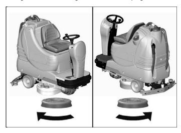
For a longer life of the brushes we suggest to invert daily their position. Whenever brushes result to be deformed we suggest to reassemble them in the same position, in order to avoid that the different inclination of the bristles causes excessive motor overload or troublesome vibrations.
